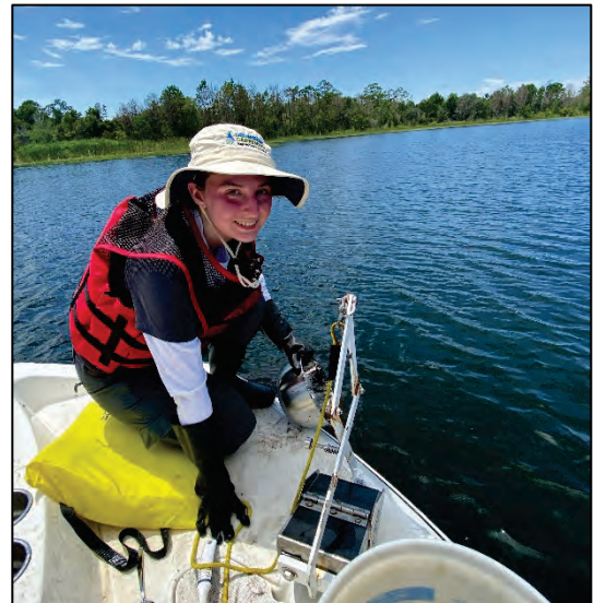
Drummond Carpenter Staff Engineer Lauren Mayou collects sediment samples to evaluate lead contamination in Big Sand Lake in Orlando, FL.
